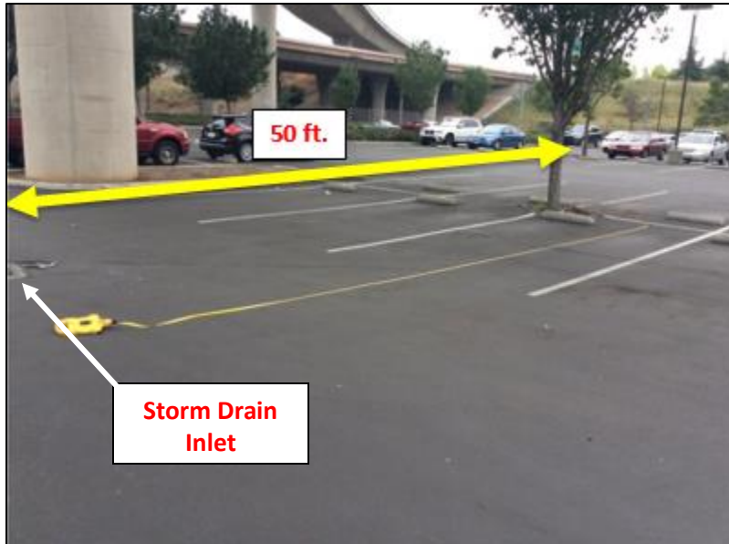
Figure 3. Example of a measuring the distance to assess from an area drain surface inlet.
